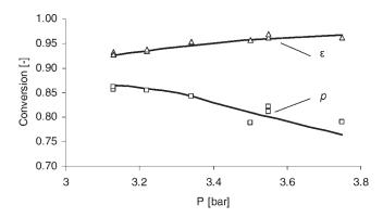
**Figure 6.**Influence of reaction pressure on conversion. Symbols: experimental values; Line: calculated.
