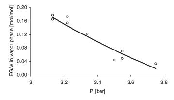
Figure 2. Effect of esterification pressure on EG/W in vapor phase. Symbols: experimental values; Line: calculated.
