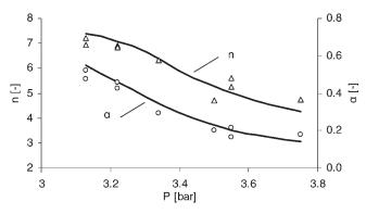
**Figure 4.** Effect of esterification pressure on n and  $\alpha$ . Symbols: experimental values; Line: calculated.
